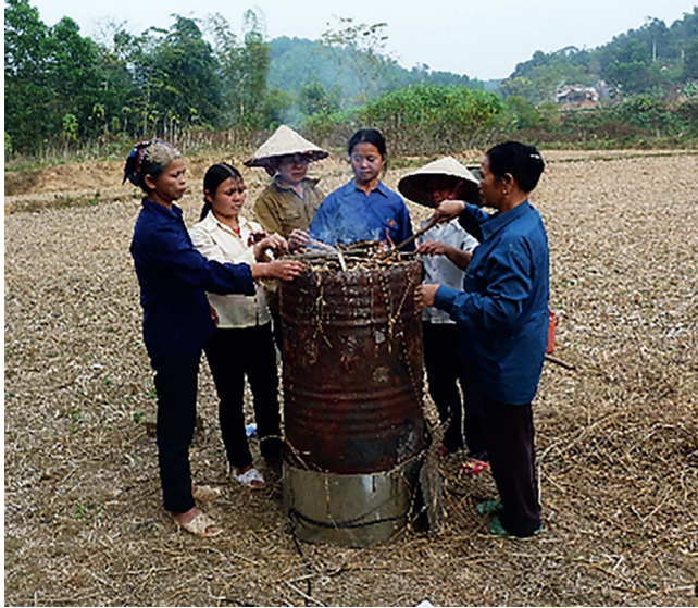
Fig. 6 Production of biochar in the field using a top lit updraft gasifier (TLUD).
